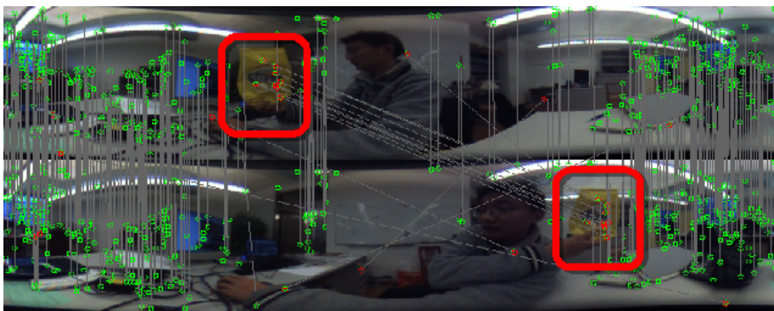
Figure 2: Result of Dynamic object detection. The red rectangles mark the detected dynamic objects from the image pair. The green circles indicate the inliers of the key-point matching, while the red ones indicate the outliers of this scene matching.
