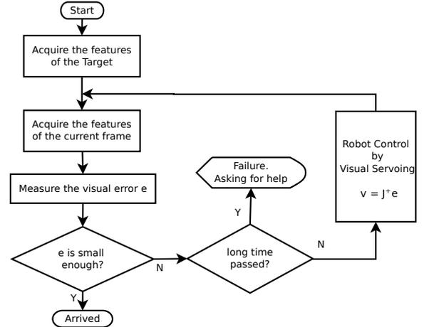
Fig. 5. The flow chart of the *pose stabilization* process
