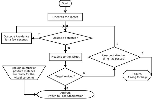
Fig. 4. The flow chart of the *general positioning* process
