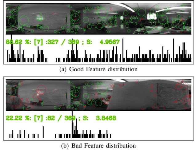
Fig. 7. Histograms of the feature distribution. There are two kinds of circles that mark the matching keypoints : green (brighter) and red (darker). The green (brighter) circles mark the matching results after RANSAC; the red (darker) circles mark the rejected matches.
