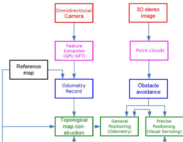
Fig. 2. The system structure
