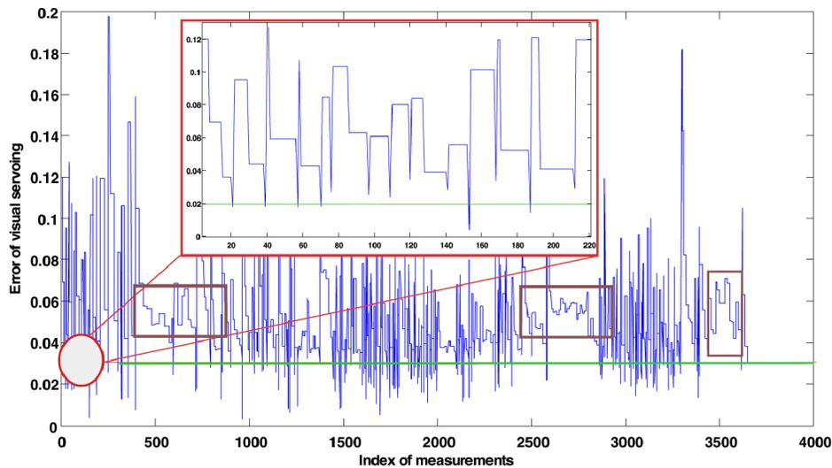
Fig. 10. Pose stabilization error vs measurement indices. The red rectangle is a magnified view of the errors in the corresponding region. The verticle axis is in the unit of visual servoing error.
