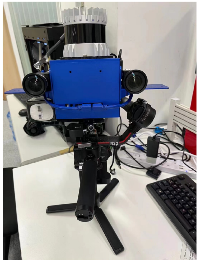
Fig. 7. Embedded system equipped with the Velodyne vlp-16 LiDAR sensor.
