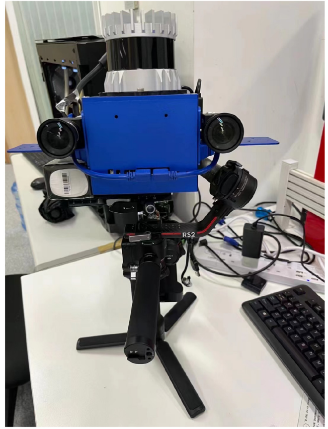
Fig. 7. Embedded system equipped with the Velodyne vlp-16 LiDAR sensor.
