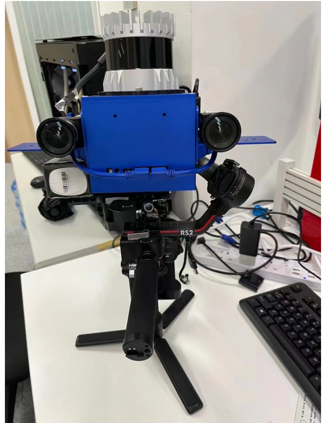
Fig. 7: Embedded system equipped with velodyne vlp-16 LiDAR sensor.
