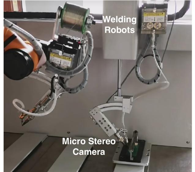
Fig. 7: Details of the employed visual welding head.
