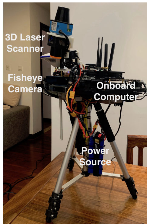
Fig. 7. The experimental platform equipped with a 3D laser scanner and a fisheye camera, along with other processing devices.
