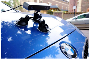
Fig. 10. Experimental set-up for acquiring stereo road images.
