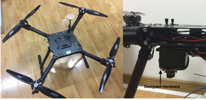
Fig. 5. Quadrotor is used for validation of the attitude estimation system involving MARG sensors and a monocular camera.
