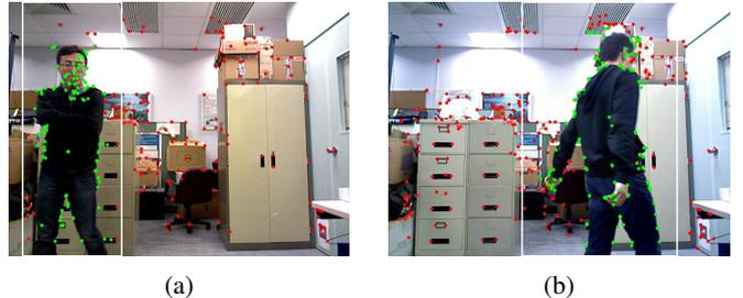
Fig. 3: The demonstration for the motion detection. In this scene, a person is walking with a normal speed in front of a static RGB-D camera. (a) and (b) show the motion detection results at different time. The feature points from the walking person and the background are coloured as green and red. The areas inside the white rectangles are the created ROIs.
