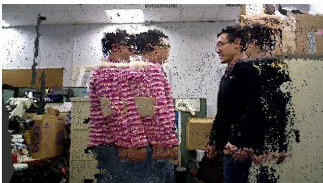
Fig. 1: The contaminated scene model built by ICP fusion. In this scene, two persons are walking in opposite directions in front of a static RGB-D camera.
