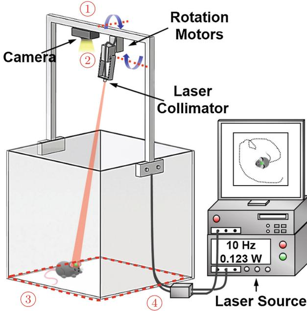
**Fig. 2.** Framework overview. ① Arbitrarily mounted camera ② Laser with Pan-Tilt ③ Target plane ④ IoT ATOM board
