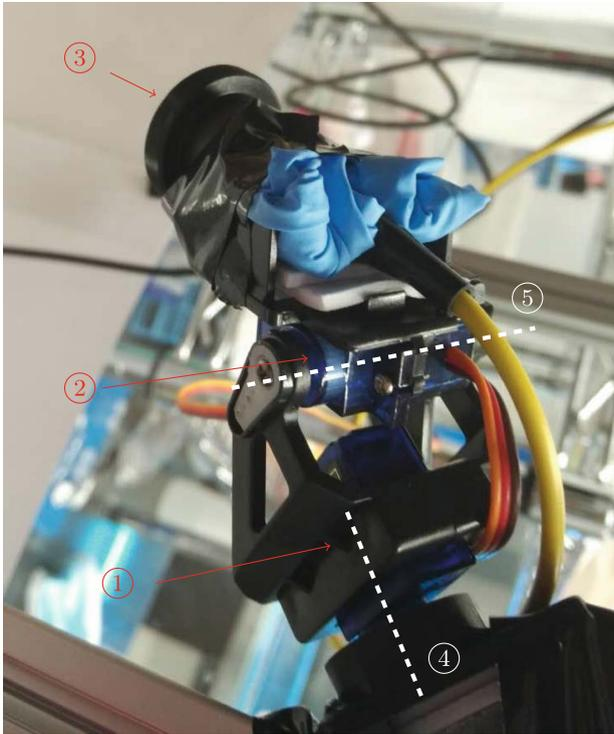
**Fig. 5.** Actuator overview. ① First servo ② Second servo ③ Laser emitter ④ Rotation axis of first servo ⑤ Rotation axis of second servo
