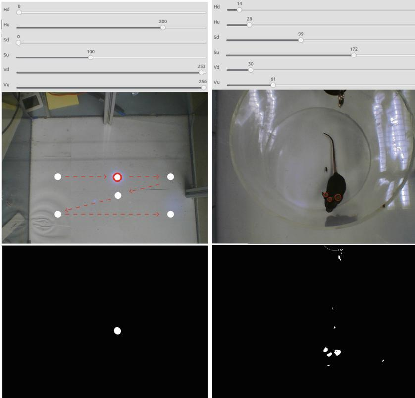
**Fig. 4.** Laser spot (left) and surgical wound of mouse brain (right) detection. Left: red circle marks the laser spot, red dashed arrow lines mark the scan path (Color figure online)
