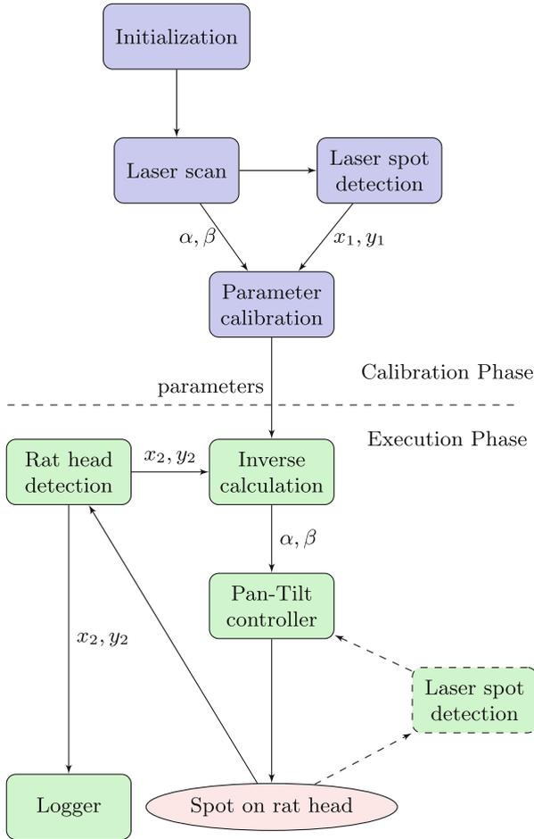
**Fig. 3.** System work flow.  $x_1, y_1$  are laser spot position,  $x_2, y_2$  are mice brain position.  $\alpha, \beta$  are the pan and tilt angle
