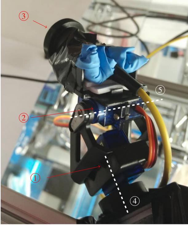
Fig. 4: Actuator overview. ①First Servo ②Second Servo ③Laser generator. ④Rotation axis of first servo ⑤Rotation axis of second servo
