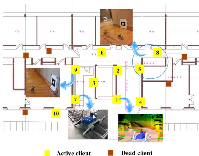
Fig. 4. A map of typical indoor environment for multi-robot co-localization (10 active robots are in a multi-hop network which has a topology as shown in Fig. 1.)
