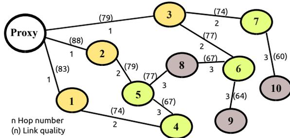
Fig. 1. A hierarchical network graph of the proposed robotic multi-hop architecture and the corresponding link quality. Nodes in the same layer are drawn in the same color, e.g.,  $v_1, v_2, v_3$  are in layer  $l = 1$ .
