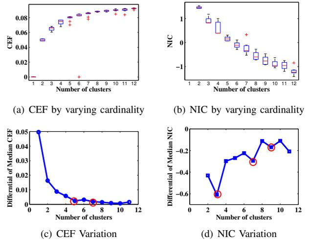
Fig. 3. Determination of cardinality of clustering. Red circles in (c) (d) marks the detected salient changes, which indicates the potential number of clusters. We could see that NIC criteria is more distinguishable in cardinality detection.
