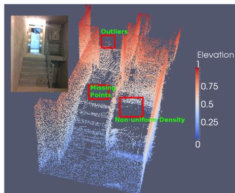
Fig. 1. Clip of a typical point-cloud and common observation noises.
