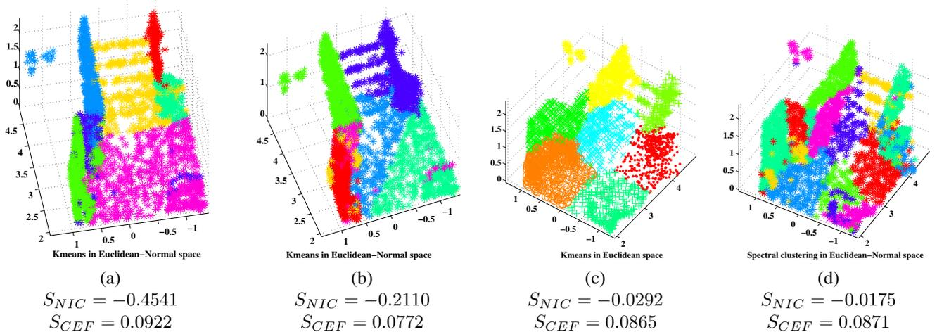
Fig. 4. Clustering results using different algorithms on the same structured dataset (after density sample: 2588 points). A lower  $S_{NIC}$ , or higher  $S_{CEF}$  indicates better result, according to definitions. We could see that  $S_{NIC}$  criterion is more informative as a assessment of the segmentation quality.
