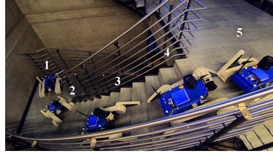
Fig. 1. NiftiBot during autonomous climbing of a curved staircase.
