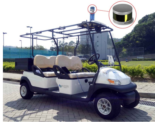
Fig. 3. Experimental Platform: Unmanned vehicle with Velodyne LiDAR VLP-16, 2D-sick LiDAR, IMU, GPS, OCCAM stereo camera and IPC (i7 intel nuc).
